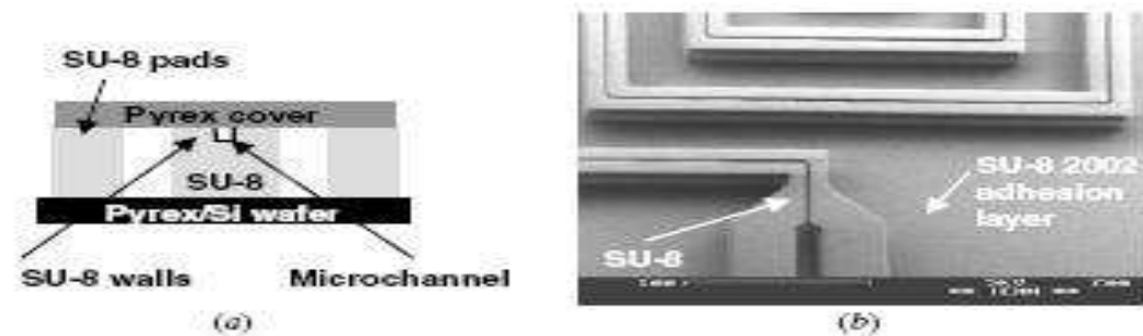
Figure 3. Microchannel formed using SU-8 walls (second generation): (a) Schematic diagram of the microchannel cross-section and (b) SEM image.
